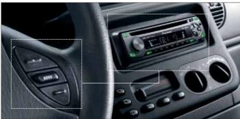
Your remote control ready Pioneer headunit can work with your car's existing built-in remote control unit, thanks to an adapter kit: infrared in the case of Pioneer's remote control ready headunits, and hard wired in the case of Pioneer headunits with a hardwired remote input (a rear mini-jack input). Several versions of adapters are also available, to suit original remote control units in most cars.\*
